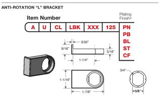
This bracket can be mounted on the top, bottom, left or rigth of the glass edge. For use with  ${\bf D},\,{\bf K},\,{\bf M},\,{\bf S},\,{\bf V},\,{\bf P}$  and  ${\bf E}$  Cam Locks.
