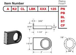
This bracket can be mounted on the top, bottom, left or rigth of the glass edge. For use with **K2** Cam Locks.
