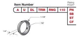
For use with D, K, K2, M, S and E Drawer/Door and Plunger Locks.
