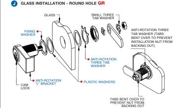
Dimension from center of hole to the edge of glass is 1-1/4"
