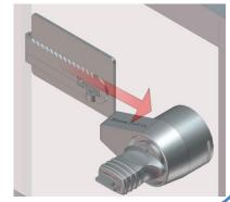
**Step 7:** Press firmly on the lock-bar plate for an additional 20 seconds. Although the adhesive should now be firmly set it is suggested to allow as much as 30 minutes to an hour of additional rest time before subjecting the locking bar to normal
