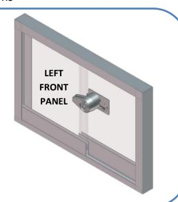
**Step 1:** Insert Bar into Ratchet Lock simulating the desired "locked position".
