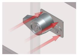
**Step 6:** Insert operating key and rotate 90° to the right to disengage the lock. Slide the lock and key assembly to the right to remove the lock (The adhesive may not be fully seated so be careful to slide directly to the right and not pull on the locking bar while removing the lock).
