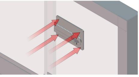
**Step 8:** Congratulations you have successfully installed the Glue-On ratchet lock bar. Slide the lock over the bar to secure the sliding doors.
