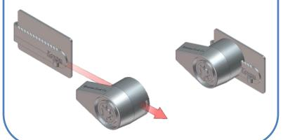
Step 2A: Test Fit the Lock on the glass. This is an important step to locate the lock when it is assembled onto the locking bar. Failure to do so may result in extra free play up to and beyond 1/8" after installation.
