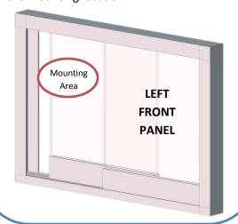
**Step 4:** Using the supplied alcohol wipe, thoroughly clean the mounting surface making sure to allow the surface to fully dry before proceeding. It will take a minimum of 5 minutes for the surface to be fully dry.
