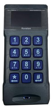
The base multi-function station can be used for key activation using a user PIN and USB or both. The activation function may be key-powered or with a battery boost supporting a larger display and keyboard backlight. With plug-in modules the station may also be used as a GSM sync station or remote key or site monitoring depending on installed hardware.
