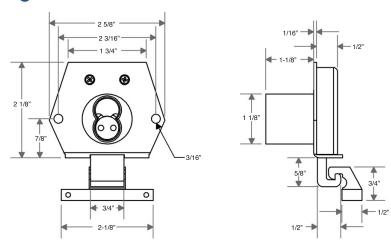
MORTISE MOUNT INVERTED INTERLOCKING SPRING BOLT
